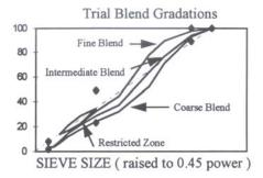
power gradation chart with control points and a restricted zone. This is used to insure a strong stone skeleton with sufficient void space for durability. The design aggregate structure is selected based on the required air voids in the total mix, voids in mineral aggregate (VMA), voids filled with asphalt (VFA), and dust proportions.
