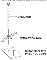
As shown at left, put the drill rod through the extraction tool and then through one of the guides on the scraper plate. Place the drill rod assembly on the test site. Step on the scraper plate. Hammer the drill rod at least 50 mm (2 in.) deeper than the desired test depth. The drill rod increments include the additional depth.
