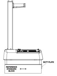
After taking a 240-sec standard count, the gauge displays the density and moisture standards (DS and MS). The gauge also displays P or F to show if the results fall within acceptable limits. The DS should be within 1% and the MS should be within 2% of the previous four standard counts. Troxler recommends that the operator keep a daily log of the standard count results, using Appendix D of the Model 3430 and 3440 Plus *Manual of Operation and Instruction* (user manual).
