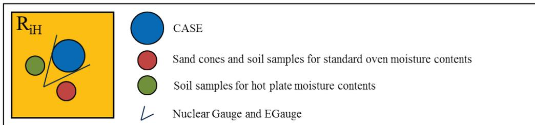
Figure 13. Testing of sand cone density following CASE, NDG, and eGauge measurements and testing of hot plate moisture content inside red ring.
