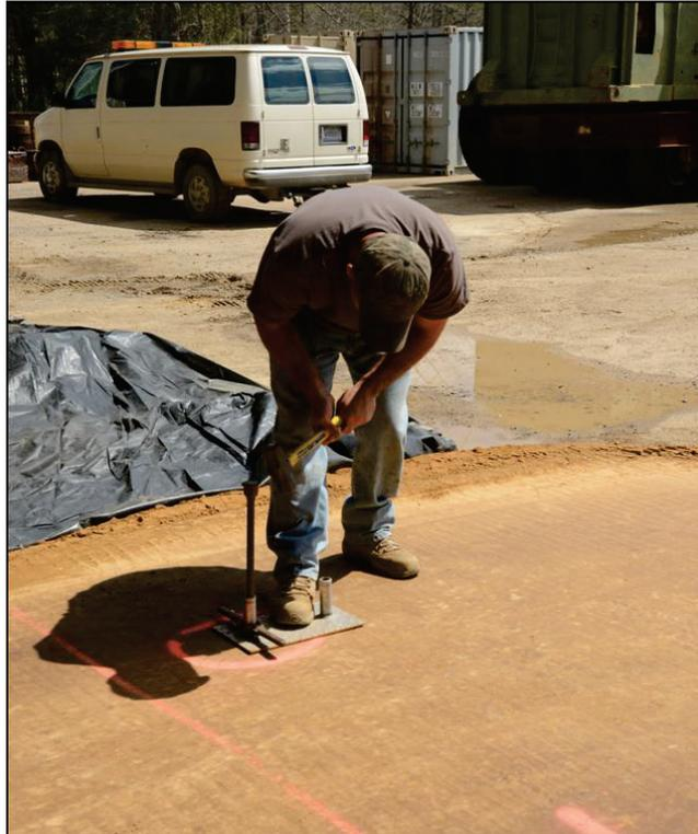
Figure 17. NDG testing alongside the CASE unit.
