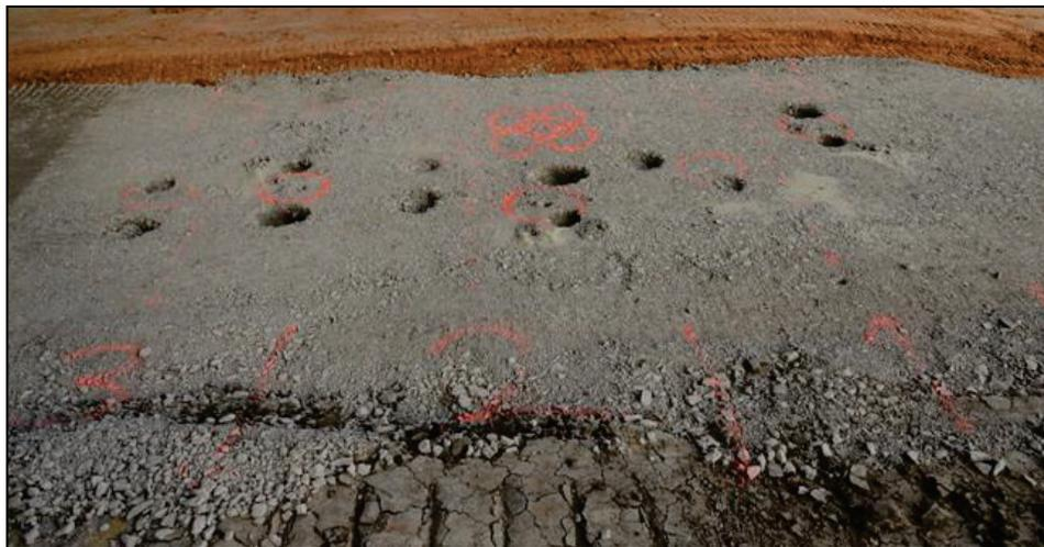
Figure 15. Cloverleaf pattern used for precision evaluation of CASE unit.
