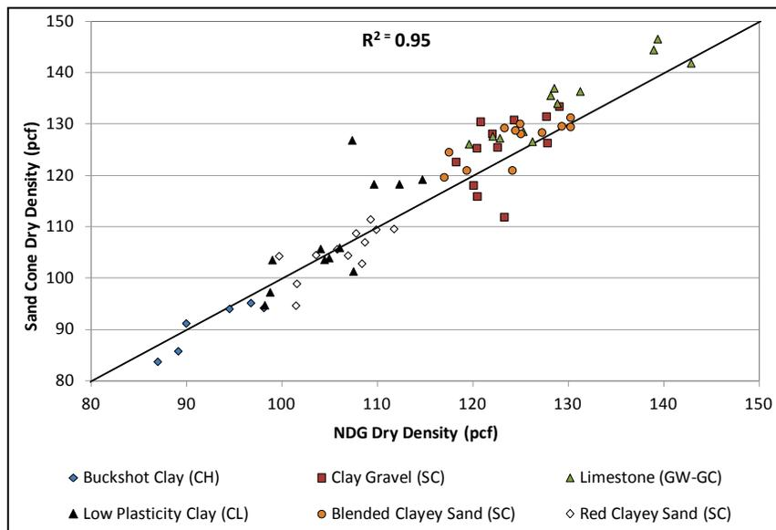
To calibrate the CASE unit for this study, the device was placed on the soil of interest in a prepared condition similar to expected during construction, in this case following the final roller pass on the first lift. A wet density and
