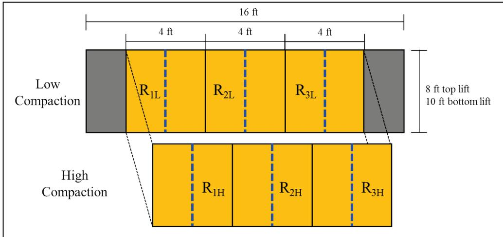
Figure 12. Typical instrument layout.
