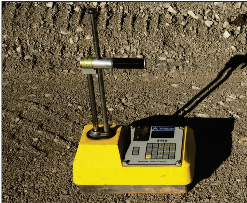
A material with a high density increases the number of collisions between the gamma photons and the electrons present in the material. Therefore, the number of photons reaching the detector tubes is reduced. Hence, the
