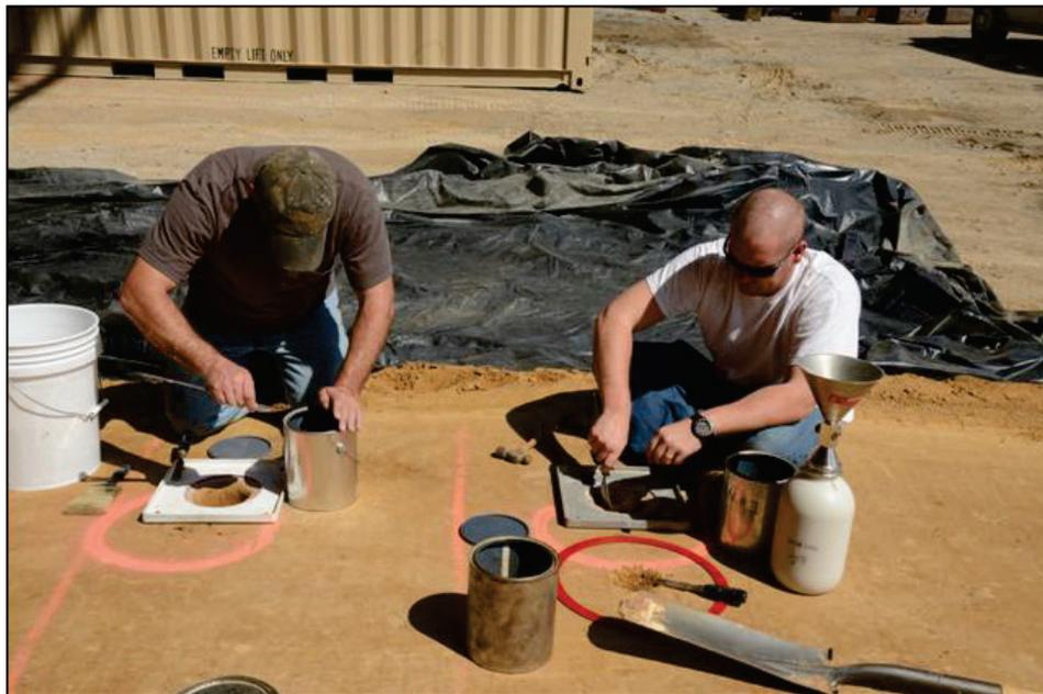
Figure 14. Posttest locations of sand cone and hot plate samples following testing on limestone test section.
