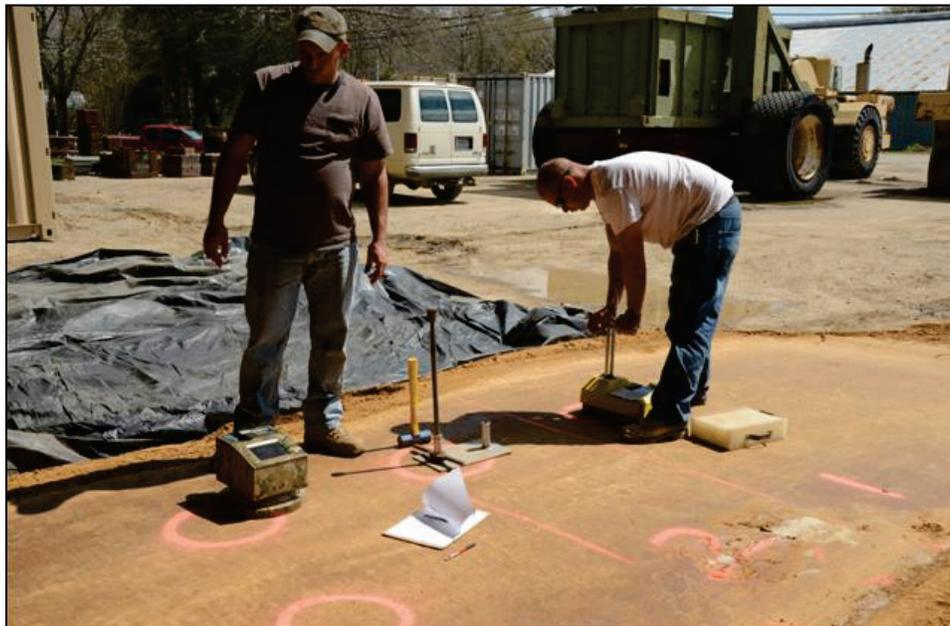
Figure 18. eGauge wet density measurement with rod at 6-in. depth.
