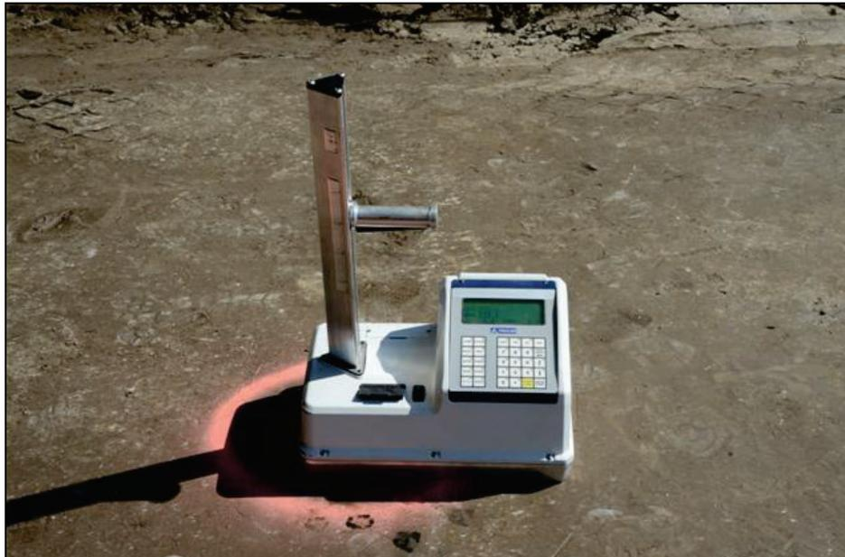
Figure 19. Insertion of the moisture probe following density eGauge testing.
